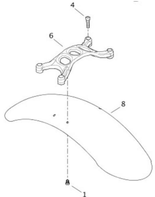
We recommend using a medium-strength screw lock (e.g. LOCTITE 243, blue) for all screws.
